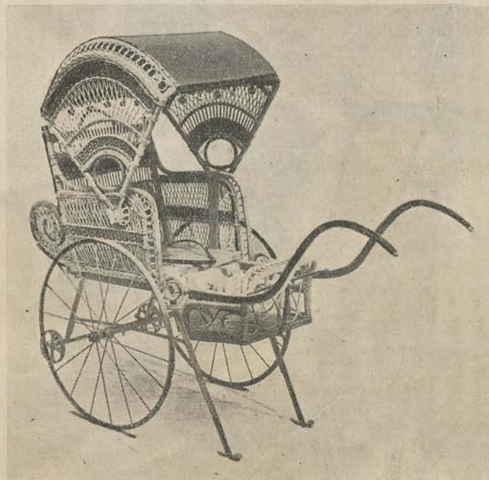
K161—Go-Cart, parcel carrier, drop extension front, ash shafts, 23in. rubber-tyred wheels, 57/6
