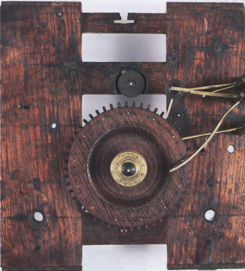
The original strike work, the wheel has been fitted with new pins.
