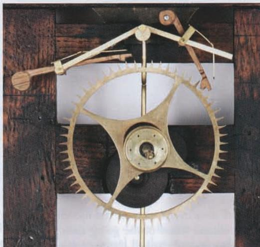
The movement with front plate removed showing the new escape wheel and Grasshopper escapement.
