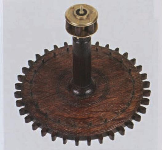
The third wheel and roller pinion with a ring of pins for the maintaining power. The rollers in all the pinion assemblies are turned in self-lubricating lignum vitae.
