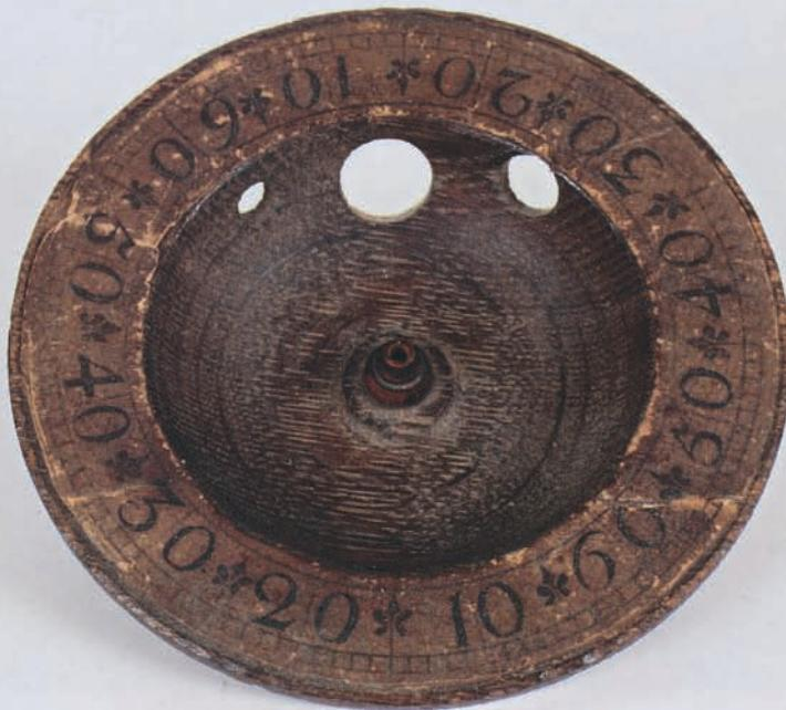
The paper facing to the date wheel is numbered, signed and dated in black ink. The paper facing on the seconds indicating wheel is also marked out in black ink for 2 x 0-60 seconds. This wheel, turned in one piece in the shape of a bowl with poising holes, acts as a flywheel for the escape wheel which rotates anticlockwise.
