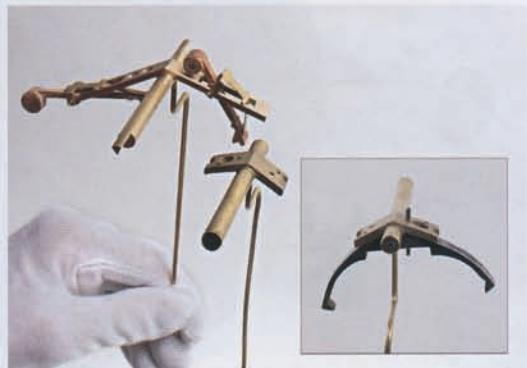
The new escapement is shown with the remnant of the original pallet arbor which had had an anchor fitted (see inset). The original escape wheel arbor was retained and the reconstruction was based upon comments in correspondence by later members of the Harrison family.
