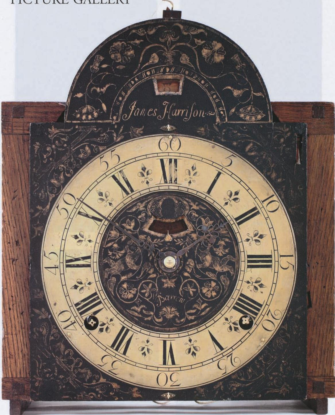
The dial board is of oak only  $\frac{3}{8}$  in. thick. The reverse is routed to only half this thickness to receive the calendar ring. The ground is black varnish, the carefully designed symmetrical decoration is of powdered gold and surely full of symbolism. The chapter ring appears to be a standard item supplied to the Harrisons. The feet have been sawn off and the ring fitted using brass pins.
