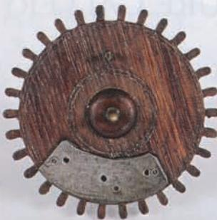
The rear of the minute wheel, showing the added lead for poising the wheel/hand assembly.
