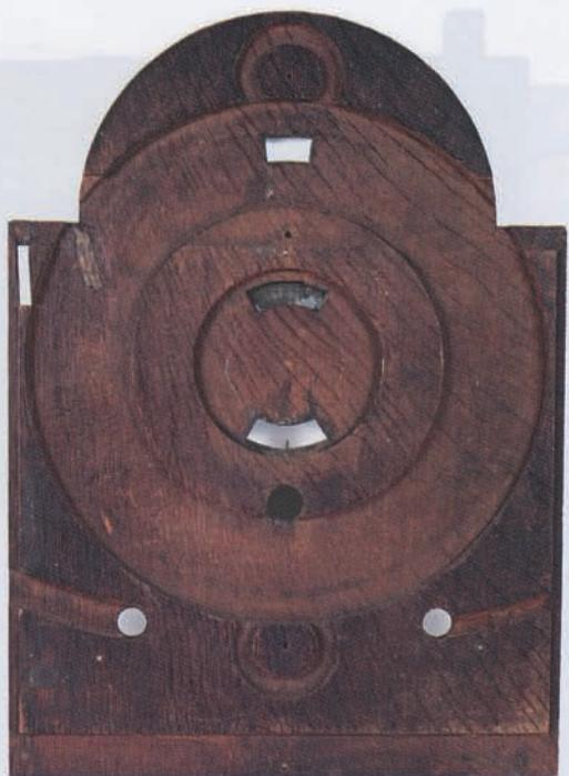
Back of the wooden dial plate with various interesting features including the unused circular cut-out at the top and the groove cut-out in error on the right for the maintaining power shutter.
