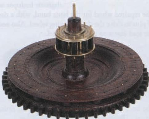
The second wheel and pinion with free running rollers to lift the hammer tail.
