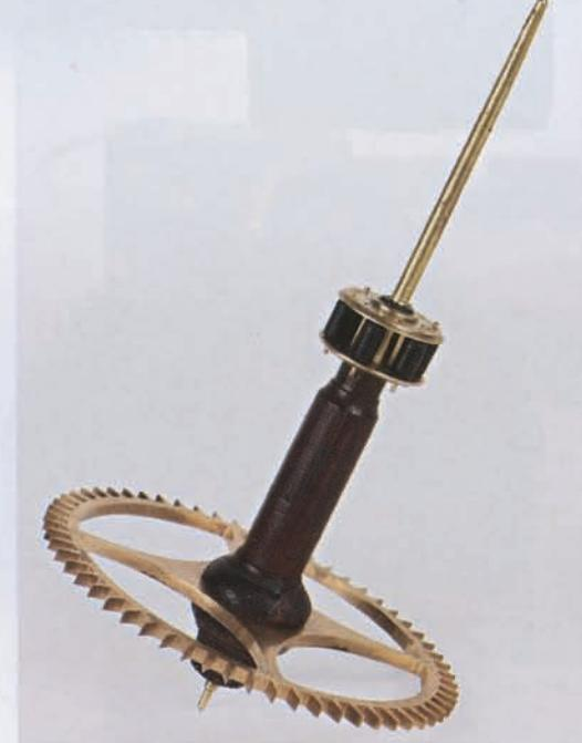
The original escape wheel arbor and roller pinion, fitted with the new escape wheel of 60 teeth. The seconds indicating disk is mounted on the extended arbor.
