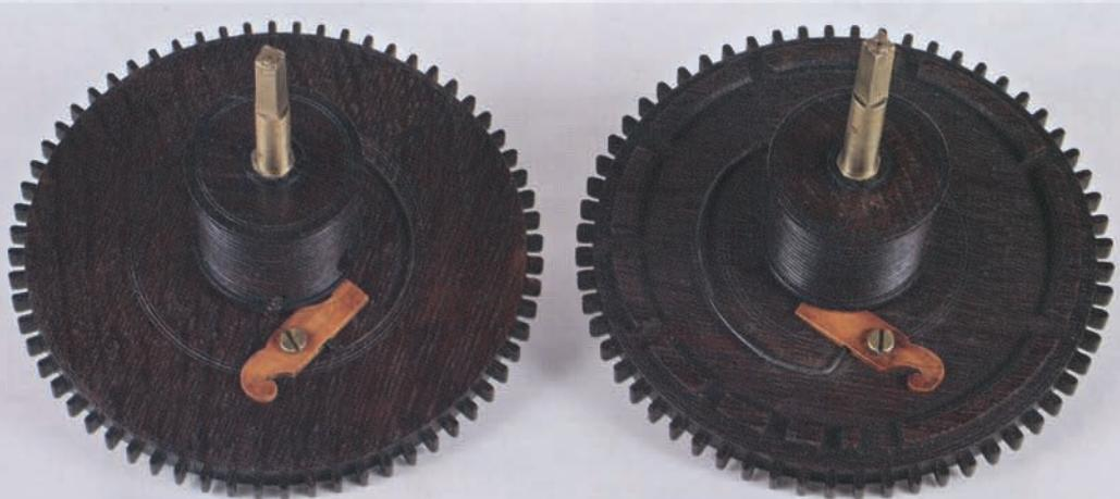
The great wheels, winding barrels with boxwood clicks and pulleys for the weight lines.
