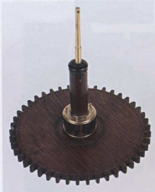
The second wheel, with wooden roller pinions held between brass discs. The motion work is driven from this wheel using the driving wheel/pinion spring mounted onto the extended brass arbor.
