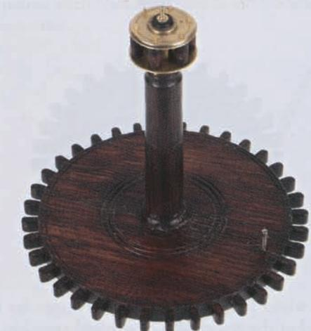
The warning wheel and roller pinion.
