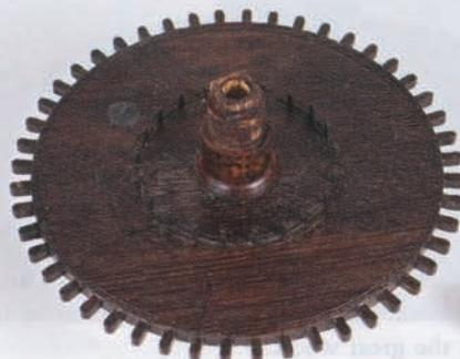
The repaired wheel for the hour hand, with a ring of pins to drive the date indexing wheel. Also note the lead insert to poise the wheel.
