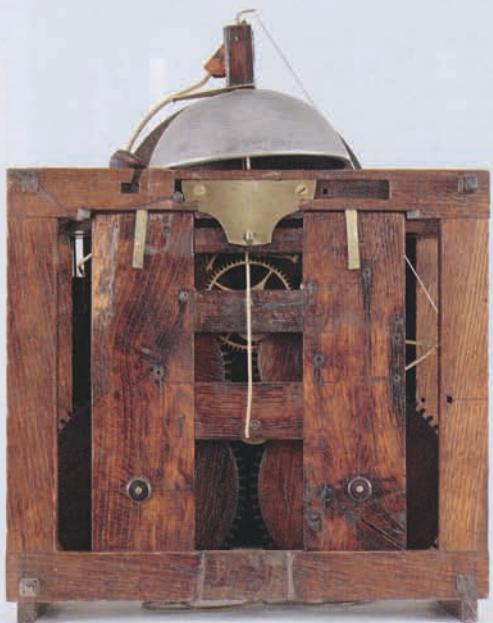
The back of the movement, with plain brass pendulum suspension bracket, a later alteration documented by Harrison.
