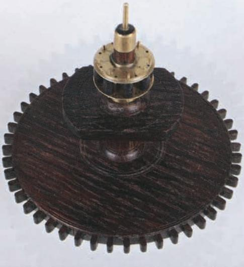
The third wheel and roller pinion with double acting cam for the striking work.
