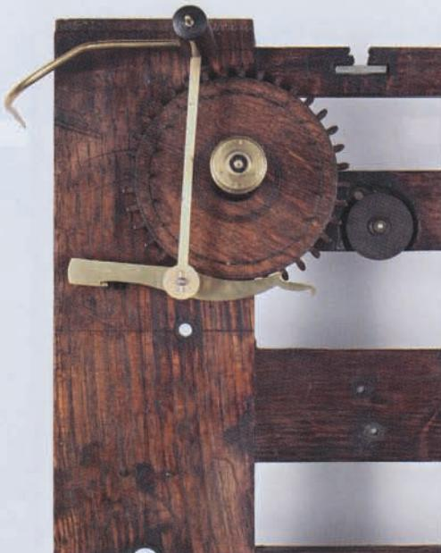
The action of the maintaining power. The wooden arbor is original, the brass work is new. An anti-friction roller for the escape wheel pivot is also visible, the second anti-friction roller is on the other side of the wooden bar.
