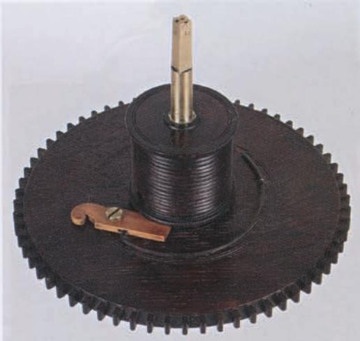
The great wheel, winding barrel and boxwood click. The wooden wheels in the clock are made in the expected Harrison fashion using teeth segments inserted into the rim of the wheel. The grain of the oak then runs the length of the tooth, to give the required strength.
