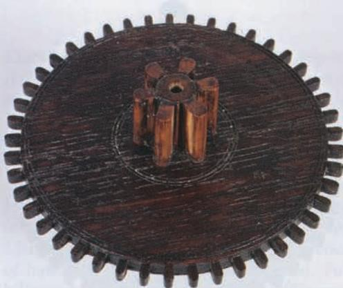
The solid boxwood pinion (not a roller pinion) with wheel for driving the motion work.
