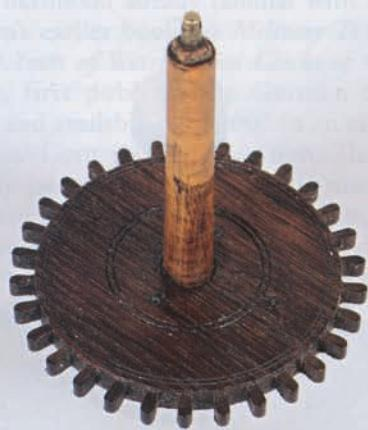
The wheel for the minute hand, driven by the wheel of the boxwood pinion/wheel assembly.
